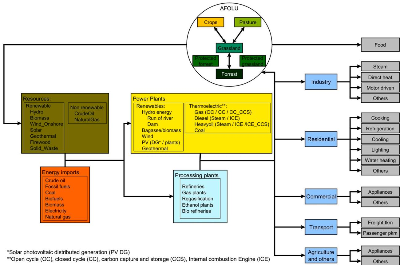
Fig. 6. Representation of the energy and land use system conversion chain in the ELENA model.
