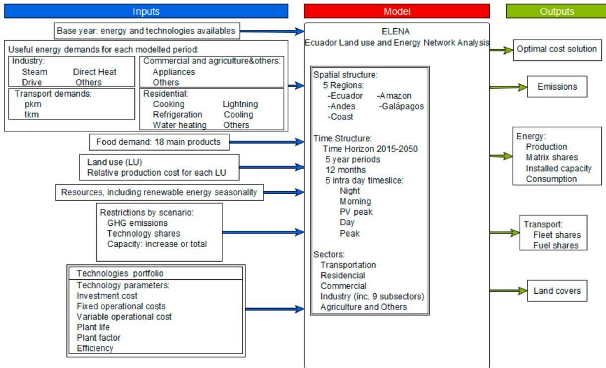
Fig. 4. ELENAs model structure, inputs and outputs.
